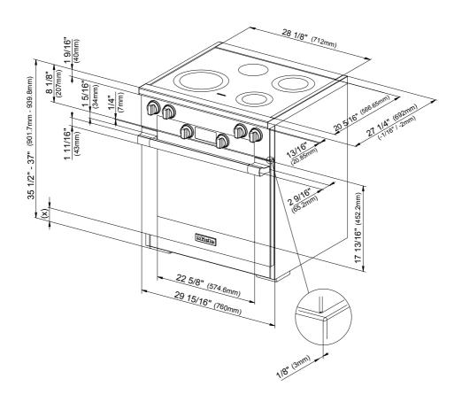
(x) = Depending on the appliance height adjustment 5" - 6 1/2" (127 mm - 165.1 mm)
