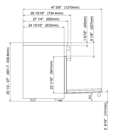
(x) = Depending on the appliance height adjustment  $5" - 6 \frac{1}{2}"$  (127 mm - 165.1 mm)
