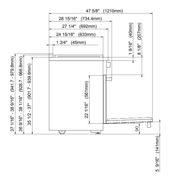
(x) = Depending on the appliance height adjustment  $5" - 6 \frac{1}{2}" (127 \text{ mm} - 165.1 \text{ mm})$
