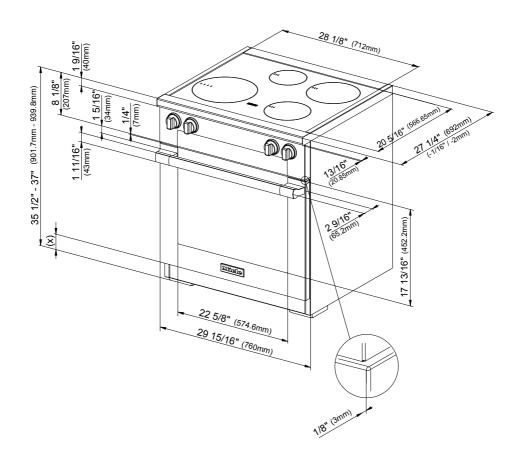
(x) = Depending on the appliance height adjustment 5" - 6 1/2" (127 mm - 165.1 mm)
