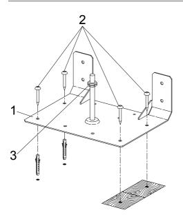
■ Screw the locking nut ③ to the bolt, see the "Installation dimensions of locking bolt" table.
