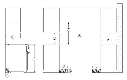
(C), (D), (E) The shaded area represents the installation area for the connections: (E) = Electrical connection, (E) = Water connection, (E) = Gas connection
