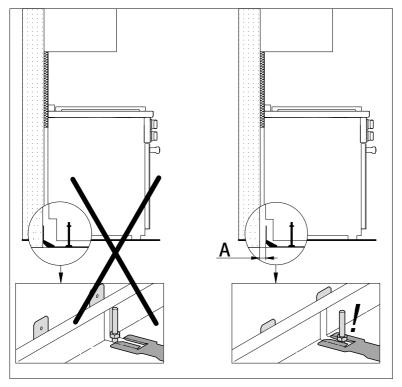
A = Distance between the rear of the range to the supporting wall
