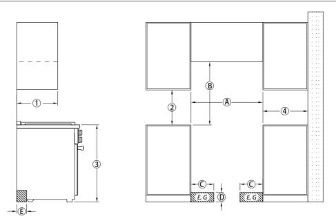
c, d, E The shaded area represents the installation area for the connections: E = Electrical connection, G = Gas connection
