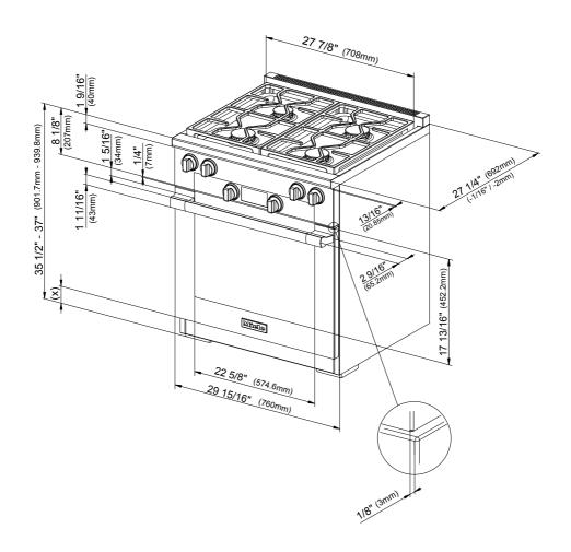
(x) = Depending on the appliance height adjustment 5" - 6 1/2" (127 mm - 165.1 mm)
