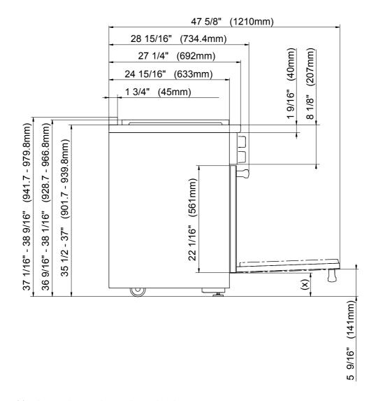
(x) = Depending on the appliance height adjustment:5" - 6 1/2" (127 mm - 165.1 mm)
