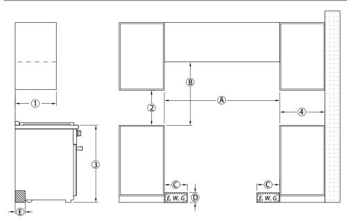
$(\hat{E})$ ,  $(\hat{E})$  The shaded area represents the installation area for the connections:  $(\hat{E})$  Electrical connection,  $(\hat{E})$  = Water connection,  $(\hat{E})$  = Gas connection
