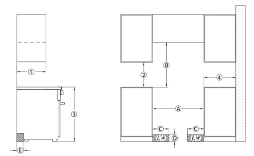
(c), (b), (c) The shaded area represents the installation area for the connections:
