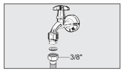
■ Connect the stainless steel hose to the water supply.
