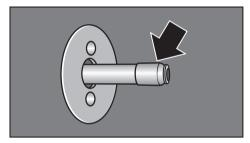
A connecting piece between the brew unit and the main dispenser is located on the inside of the door.
