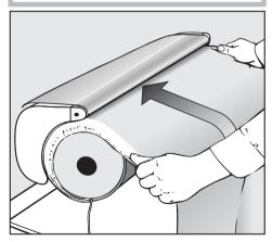
Press the foot pedal and "iron" the new cloth all the way around.
