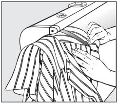
The collar is ironed on both sides using the left hand end of the roller. Stop ironing when the button comes to the heater plate. Then turn down the collar and press lightly, holding taut.
