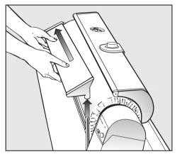
Lift the feed board out of the right-hand holder, then pull it outward toward the left of the roller.
