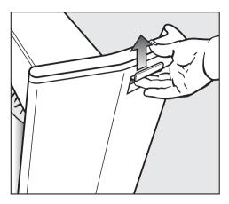
Hold the ironing table and release the catch, located on the right-hand side at the back, underneath the ironing table.
