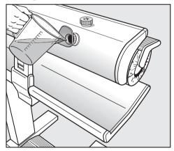
Before turning on the iron, and with the roller in the up position, fill the water reservoir to the lower edge of the spout with **tap water** approx. 1 <sup>1</sup>/<sub>2</sub> pints (0.8 I).
