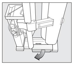
Keep the strut in a safe place. It will need to be attached each time you transport the appliance.
