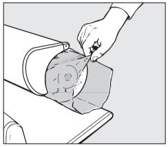
The protective dust cover can now be pulled off. The adhesive film supplied with iron can now be placed around the temperature selector.
