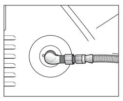
■ Secure the flexible metal gas line connector to the adapter.
