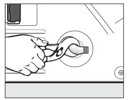
At the end of the dryer's gas connection hand screw on the <sup>3</sup>/<sub>8</sub>" NPT elbow.
