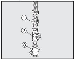
■ Connect the flare union adapter, ①, to the pressure tapping plug, ②, originally installed on the gas shut off valve, ③.
