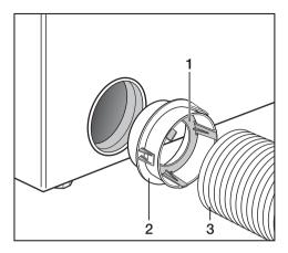
■ Install the exhaust hose **3** in the dryer using the adapter **2** and the restriction insert **3**.
