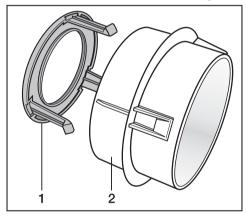
■ Place the restriction insert 1 into the adapter 2.
