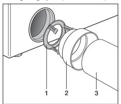
■ Plug the restriction insert 1 into the gray adapter without clips 2 and connect the pipe 3.
