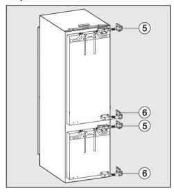
■ Clip the spacers ⑤ and ⑥ onto the top and bottom hinges.
