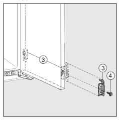
■ Screw the supplied mounting brackets ③ into the pre-drilled holes in the appliance doors using a hex screw ④.
