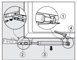
■ Carefully push the tension spring ① outward with a screwdriver.
