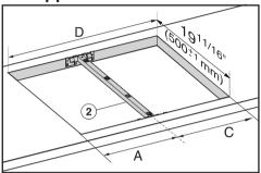
For the installation of **two appliances** the width of the countertop cut-out D is the sum of A and C.
