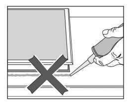
The appliance **must not** be permanently sealed into the countertop when installed. The sealing strip under the edge of the appliance provides a sufficient seal for the countertop.
