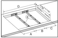
For the installation of **three appliances** the width of the countertop cut-out D is the sum of A and B and C.
