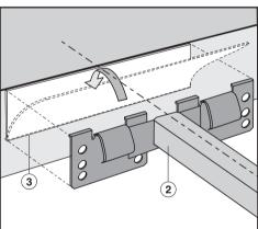
■ Position and attach the spring clips
