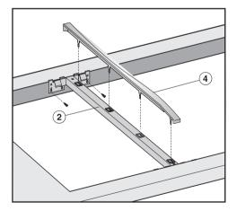
■ Insert the cover ④ into the holes in the support bar ②.
