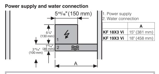
Install a pressure limiting device and water hammer arrester for inlet water pressures exceeding 80 psi.(Refer to Uniform Plumbing Code, Sections 608.2 and 609.10) Never install or operate where inlet water pressure may exceed 120 psi.
