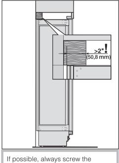
It possible, always screw the wooden beam to existing studs.
