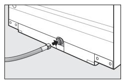
position the device in front of the niche and push the stainless steel tube through the hose guide at the back of the unit.
