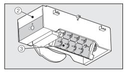
An ice cube tray ③ where ice cubes are produced is integrated in the ice cube maker ②.
