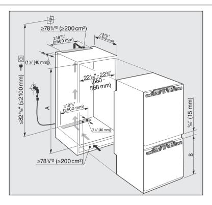
Before installation, ensure the building-in niche is the correct size. The specified ventilation cross-sections must be adhered to in order to ensure the correct functioning of the appliance.
