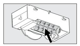
The ice cube tray ② is **not** removable and can only be cleaned when in place. You can therefore place the ice cube tray in the cleaning position.
