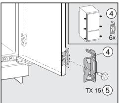
■ Screw fixing bracket ④ using hex screw ⑤ to the pre-drilled holes in the appliance door. Using the pre-drilled holes in the appliance door, secure a second pair of fixing brackets ④ in the handle area of the door.
