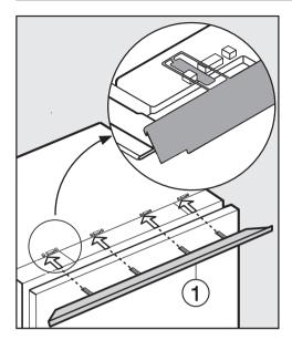
■ Fit the straps of the compensation strip ① into the strut seats from the front.
