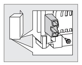
Undo the screw and remove the spacers.
