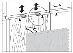
**Tip:** Push installation aids ② together with the cabinet front up to the height of the adjoining unit cabinet doors.
