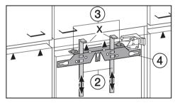
■ Remove the nuts ③ and take the mounting bracket ④ off together with installation aids ②.
