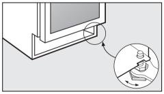
Use the provided wrench to adjust the feet as needed.
