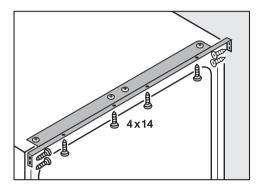
Using the fixing strip and screws, secure the appliance into place.
