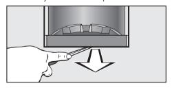
Carefully remove the drip tray using a screwdriver if necessary. Once the drip tray has been removed, the four metal strips can be used to align the Ice/Water Dispenser.
