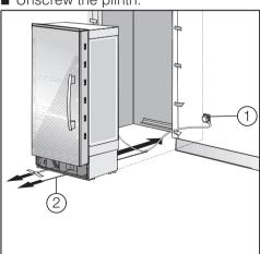
To protect the corners of the installation space, attach edge protectors where needed (not included). ■ Plug the appliance into the power outlet ①.
