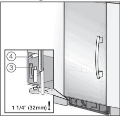
The height-adjustable feet at the front and rear can all be adjusted from the front:
