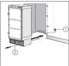
To protect the corners of the installation space, attach edge protectors where needed (not included). ■ Plug the appliance into the power outlet ①.
