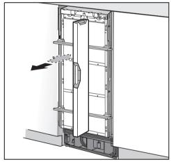
Align the appliance again using a level.
