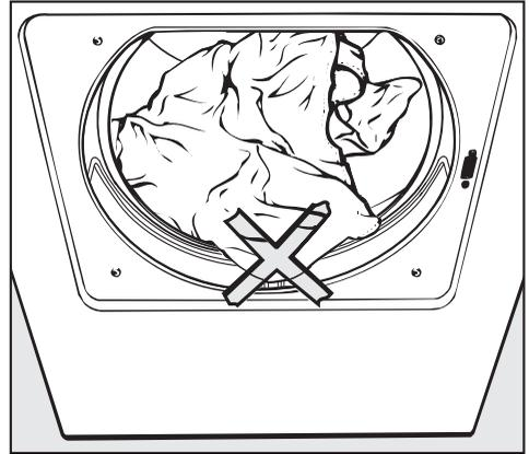
To prevent fabric damage, check that laundry is not caught in the closed door. Do not use softener sheets in this dryer. Silicates contained in these sheets could cause the dryer to overheat.
