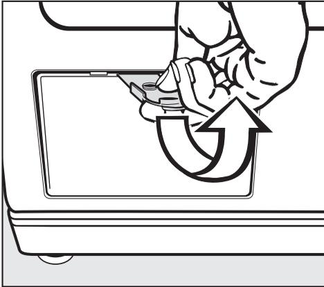
The hooks at the side will prevent the panel from falling off.
