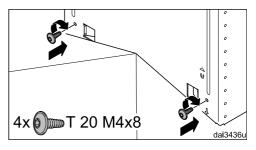
Secure the hood with the screws supplied.
