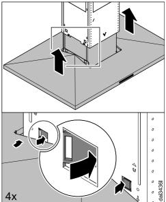
■ Hang the ventilation hood canopy on the chimney by pushing the canopy up into the installation frame and pressing the retaining clips into the openings as shown. Ensure the controls are at the front.
