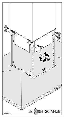
■ Raise the canopy to the desired height and secure it with the screws.
