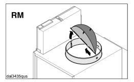
With vented mode (AE) insert the non-return flap in the exhaust socket if your ducting system is not equipped with one. Recirculation mode (RM) does not require the non-return flap to be inserted. If there is one present, it should be removed.
