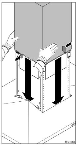
■ Hold the chimney securely, bend back the retaining tabs and carefully lower it.
