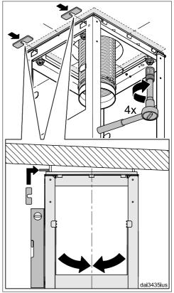
Align the installation frame and secure it with the screws. The spacers, which were removed from the spacer frame at the start, can be used to align the hood vertically.
