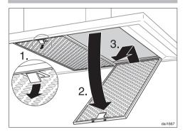
■ To remove the grease filter pull the locking clips forward, lower the filter down 45°, unhook it at the rear, and take it out.
