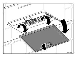
■ To remove a grease filter, release the locking clip. Then, open the filter to a 45° angle, unhook it, and remove it from the hood.
