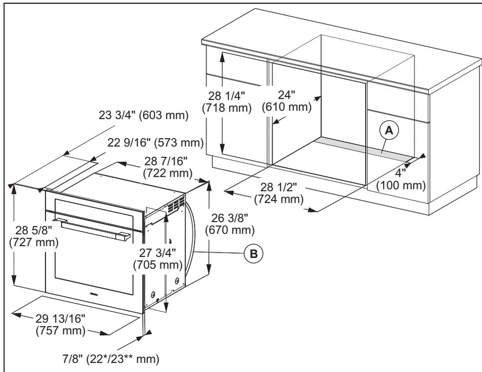
**(A)** Cut-out (4" x 28" / 100 mm x 720 mm) in the bottom of the cabinet for power cord and ventilation
