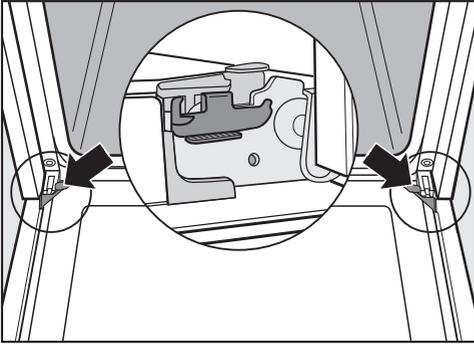
The door is connected with brackets on each door hinge. Before the door can be removed the hinges must first be unlocked.
