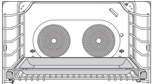
You can also place the universal tray directly on the FlexiClips with wire rack.
