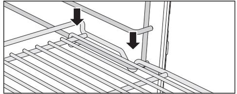
Always place the wire oven rack on the runner with the notch facing down.
