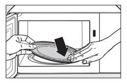
Remove the turntable and wash it either in the dishwasher or by hand with a liquid dish soap and water.
