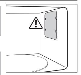
Do not remove the plate cover to the microwave outlet in the oven interior or the film that covers the inside of the door.
