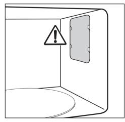
Do not remove the plate cover to the microwave outlet in the oven interior or the film that covers the inside of the door.
