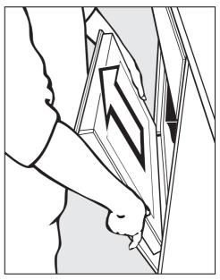
■ Holding the door securely at both sides, lift it straight upwards.
