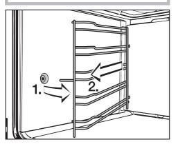
■ Pull the runners out of the holder (1.) at the front of the oven, and then pull them out of the oven (2.).
