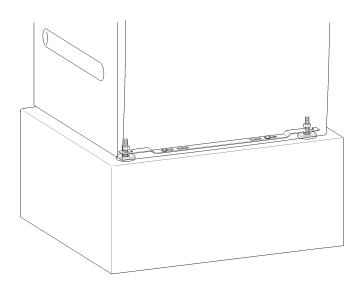
Use the supplied mounting bracket to attach the two front mounts of the appliance to the floor. The fixing material is designed for a dowel attachment to concrete flooring.
