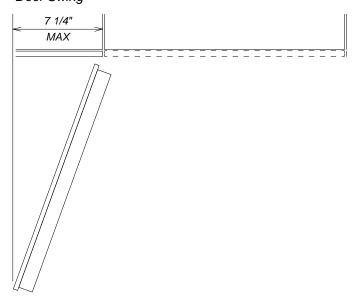
**NOTE**: Additional space needed depending on the thickness of front panels and handle used.
