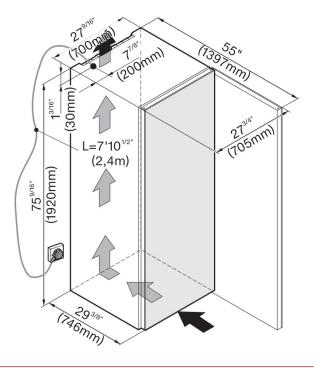
DIMENSIONS Width: 27 <sup>3</sup>/<sub>4</sub>" Height: 75 <sup>9</sup>/<sub>16</sub>" Depth: 29 <sup>3</sup>/<sub>8</sub>"
