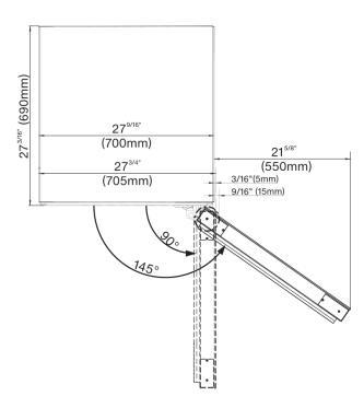
Note: Door hinge is interchangeable, see manual for further instructions Freestanding unit - does not require cabinetry
