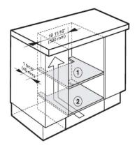
To ensure that the Combi Steam Oven has adequate ventilation, the following cut-outs measuring 19 11/16" x 1 9/16" (500 x 40 mm) must be made:
