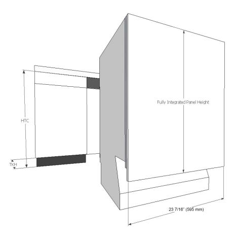
Width: 23 7/16" (595 mm) in all Cases Thickness: 3/4" (19 mm) in all Cases Height: Determined using the following
