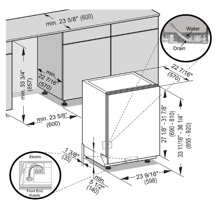
**Drain** - 4 ft 11 in (1.5 m) flexible drain hose.
