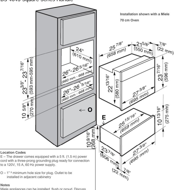
E – The drawer comes equipped with a 5 ft. (1.5 m) power cord with a three-prong grounding plug ready for connection to a 120V, 15 A, 60 Hz power supply.
