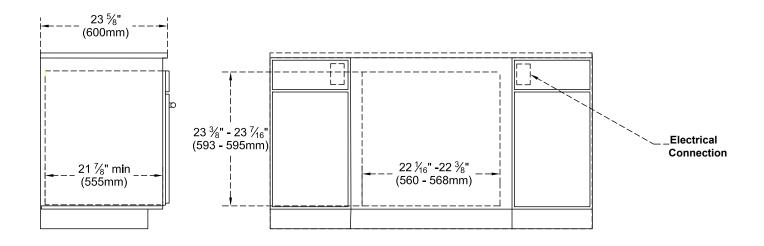
Warming drawer installation is typically placed under another unit such as a speed oven, steam oven or coffee system.
