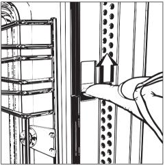
Raise the small door found on either side of the inner edge of the oven.
