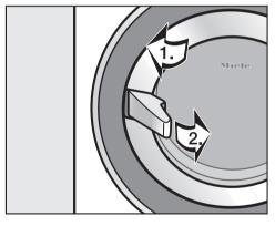
■ Close the drum door (1.). Press the door firmly shut then lock the handle into position(2.).
