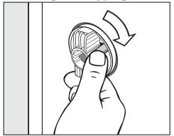
■ Release the catch and turn the left hand shipping strut clockwise by 90°.
