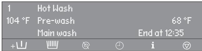
The second display line, here Pre-wash, shows the wash water temperature.
