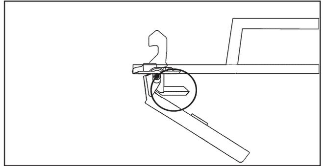
The door handle has lost its function. The door cannot be opened or closed.
