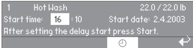
The display shows the current time of day and date. The entry field is highlighted for hours.
