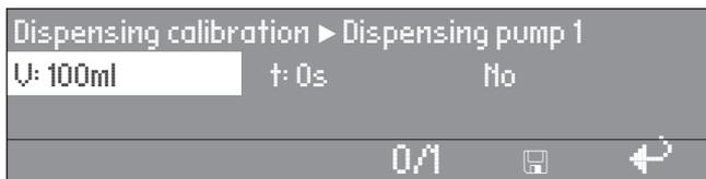
The dispensing amount can be adjusted in 1 ml increments from 0 to 999 ml.
