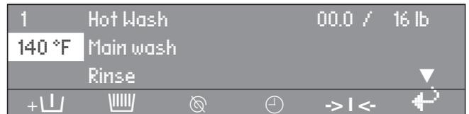
If there was still laundry in the drum when the weight display was reset, the display shows:
