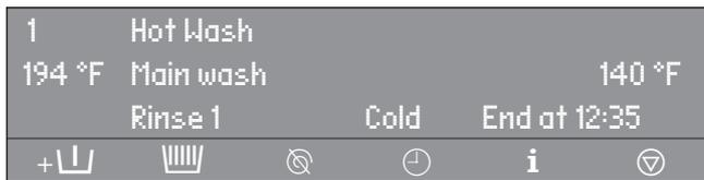
If the program block Pre-wash has ended, the 2nd line in the display shows the program block Main wash with the current wash water temperature. The 3rd line shows the following program block, here Rinse 1.
