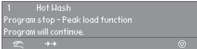
When the peak load function ends the program will continue automatically.
