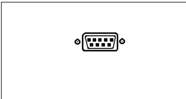
A serial interface is located at the rear of the washer to connect the machine to a PC (Personal Computer).
