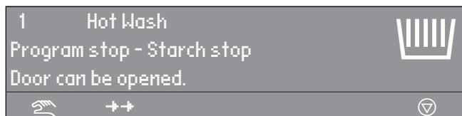
"Program stop - Starch Stop" flashes in the display when it is time to add starch to the laundry.
