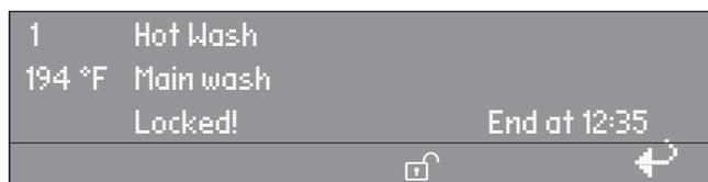
The display shows that the program is locked if the
