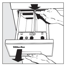
Pull out the detergent dispenser drawer until a resistance is felt.
