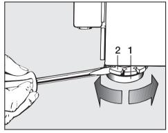
Holding foot 1 securely with a pipe wrench use a screwdriver to turn counternut 2 in a clockwise direction until it is held firmly up against the housing.
