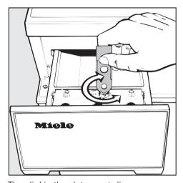
The dial in the detergent dispenser can be set as a water hardness reminder. Use the spatula (supplied for opening the drain filter panel).
