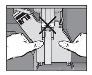
Push the brew unit in the track straight into the appliance without pressing "PRESS" until it clicks into place.
