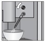
Place a 1 liter container below the steam nozzle and turn the steam selector counterclockwise. The coffee system will begin the automatic descaling. The display will read:
