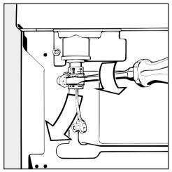
Loosen the hose clamp at the drain outlet at the lower left rear of the machine and remove the rubber plug.
