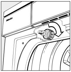
Unscrew the plastic blub cover located inside the drum and above the door (see illustration).
