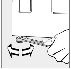
The machine can be leveled by turning the legs clockwise or counterclockwise as necessary. \* These items are available from the Miele Parts Dept.
