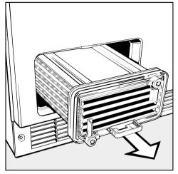
Pull out the heat exchanger.
