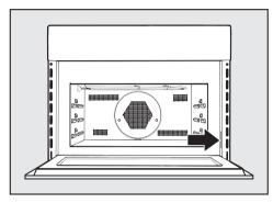
When contacting Technical Service please quote the serial number and model of your oven. This information is visible on the silver data plate along the right side of the oven.
