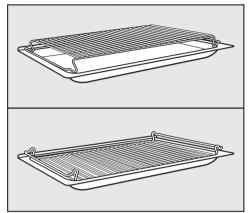
Depending on the oven function and food height, the combi rack can be used right-side-up (upper illustration) or upside down (lower illustration). This assures an optimum distance to the upper heating element.
