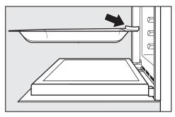
These trays are suitable for all microwave oven functions. They have non-tip safety notches which prevent them from being pulled out completely.
