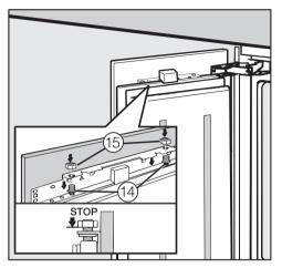
Open the door and hang the custom door with the mounting frame over the threaded bolts <sup>(1)</sup>.
