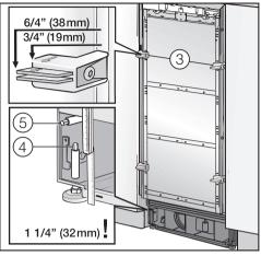
The installation aids ③ on the appliance door have been designed for custom door thicknesses of 3/4" (19 mm) and 1 1/2" (38 mm).
