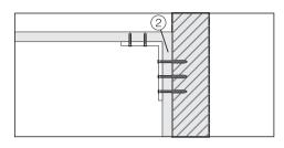
Two anti-tip brackets are recommended for each appliance. For side-by-side installations 4 brackets are recommended
