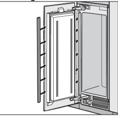
To mount the cover strips on both sides of the door, click them into place from bottom to top, into the gap between the appliance door and the custom door.
