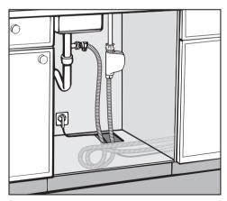
■ Make a 2" x 4" (5 x 10 cm) cut out in the side or bottom of the cabinet adjoining the dishwasher. This cut out is necessary for connections to pass through. Make certain that there are no rough edges that could damage the power cord or hoses. If metal cabinets are used, place the supplied rubber grommet around the edge of the opening before passing the cable through.
