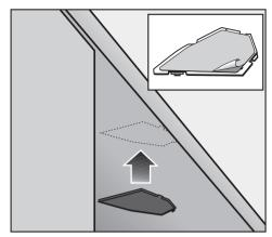
■ Line up the black reflector holder with the tracing and press into place.
