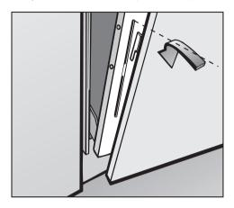
■ Place the lower mounting clips into the slots of the dishwasher door as shown in the illustration.
