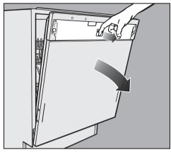
■ Grip the T shaped opening with a finger and pull the door open.
