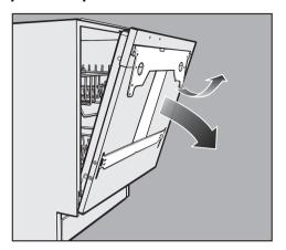
■ Gently pull on the upper portion of the mounting bracket until the door latch releases (small arrow).
