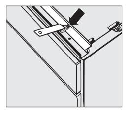
■ Insert the tab of each bracket into the guide holes on top.
