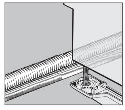
Slide the machine into the opening, making sure the electrical cable and hoses can reach their connection points without kinking.
