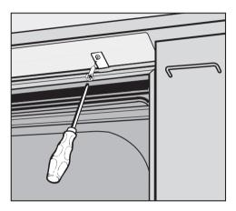
■ Using flat head screws, secure the dishwasher to the countertop by screwing through both the mounting bracket and the steam deflector.
