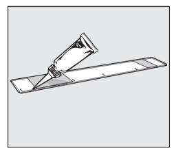
Squeeze the supplied silicone sealant along the groove of the deflector.
