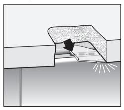
The left side of the reflector and the optic indicator in the the control panel must line up for the reflector to work.
