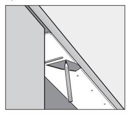
With the reflector cut out left and frontward, align the steam deflector with the front edge of the counter.
