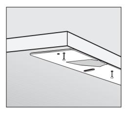
■ **Center** the steam deflector in the opening for the dishwasher and align with the lower front edge of the countertop.
