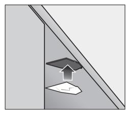
■ Press the optic indicator reflector into the reflector holder.
