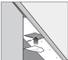
■ Press the optic indicator reflector in place.
