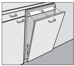
The "T" shaped hanger behind the door handle should fit easily into its respective hole.
