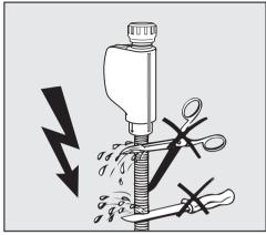
MARNING - Elcetrical Hazard Do not cut the intake hose. If the hose is cut, the dishwasher will not work. There will be a water leak and you could be injured. If the hose is too long, coil it neatly and place it behind the machine.
