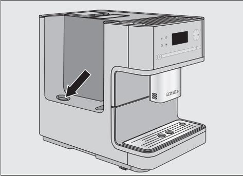
Particles in the water can collect on the fine mesh in the filter. Therefore the stainless steel filter should be checked monthly for soiling.
