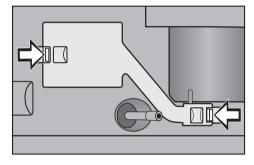
Unlock the cover for the milk pipework by pressing in the two brackets on the left and right.
