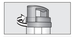
To rinse the pipework in the lid of the stainless-steel milk container, fill the large cleaning container to the "max." mark with **lukewarm** water to dissolve the cleaning agent. Fit the lid of the stainless-steel milk container into place on the large cleaning container. Hang the cleaning container in the
