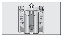
■ Turn the cover around, slide the insert upward and out, and clean both parts thoroughly.
