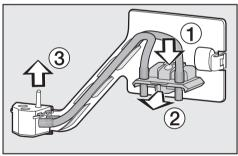
Do not pull the milk hoses off the retainers. This may cause the milk pipework to leak.
