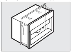
■ If there is no sealing strip around the installation recess, stick the Miele sealing strip onto the appliance from the back before putting it into the recess. Sealing strips are available from Miele.
