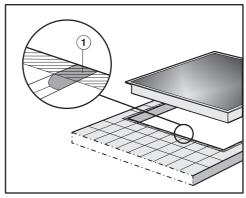
The grouting ① and shaded area under the appliance frame must be flat and even so that the frame will lie evenly and the sealing strip under the edge of the upper part of the appliance can provide an adequate seal against the countertop.
