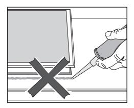
In case a disassembly is required, the appliance must not be permanently sealed into the countertop when installed. The sealing strip under the edge of the appliance provides a sufficient seal for the countertop.
