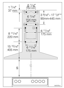
When installing a custom back wall with pre-drilled holes, please refer to the drilling distances in the drawing above (screws Ø 3/16" (5 mm)).
