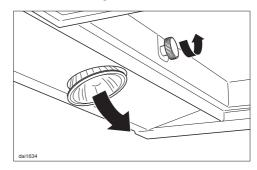
Turn the bolt counterclockwise as far as it will go. The halogen lamp will then drop down towards you.
