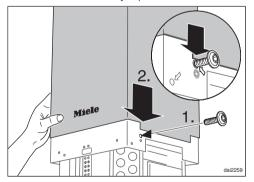
■ Secure the chimney using the previously removed safety screw.
