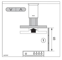
■ To create a larger distance "S" from the cooking surface ①, raise the canopy until the proper safety distance is reached.
