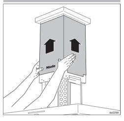
■ Push the chimney upwards.
