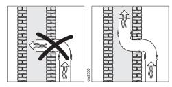
If the exhaust is ducted into an inactive flue, the air must be expelled parallel to the flow direction of the flue.
