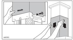
■ Remove the safety screw and lower the chimney.
