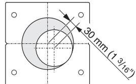
The exhaust connection in the ceiling plate is not secured in the center. This makes installation possible if the connection in the ceiling is not centered above the cooktop. A max. variance of 1 3/16" (30 mm) in any direction is possible.
