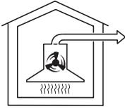
The ventilation hood works by **air extraction**. The air is drawn in and cleaned by the grease filter and directed outside.
