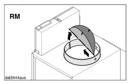
With vented mode (AE) insert the non-return flap in the exhaust socket if your ducting system is not equipped with one. Recirculation mode (RM) does not require the non-return flap to be inserted. If there is one present, it should be removed.
