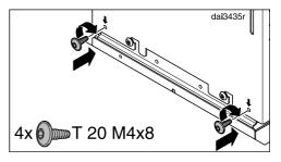
Secure the hood with the screws supplied.
