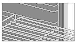
Always slide the wire oven rack into the rails on the shelf runner with the catches facing down.
