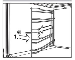
■ Pull the front of the shelf runners out of the holder (1.) and remove the runners from the oven (2.).
