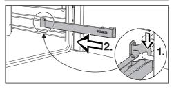
Hook the FlexiClip runner onto the front of the lower rail of a side runner (1.) and then push it along the rail into the oven compartment (2.).
