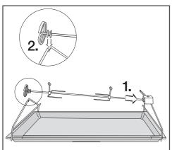
■ Insert the pointed end of the spit into the rotisserie (1) and place the roller in the holder (2) as illustrated.
