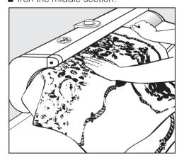
■ Fold in half with unironed edges together and place over the left end of the roller with the ironed middle section hanging over the edge to prevent creasing. Then pass both sides of the non ironed sections through the rotary iron.
