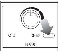
The rotary iron is turned on and off with the "0-1" button.
