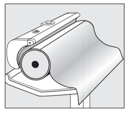
■ Completely unwind the cotton padding attached to the roller and let it hang down smoothly.
