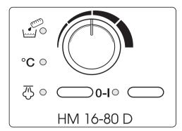
Use the **I-0** button to turn the rotary iron on and off.
