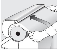
■ Press the foot pedal and "iron" the new cloth all the way around.
