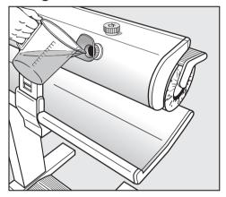
■ Before turning on the iron, and with the roller in the up position, fill the water reservoir to the lower edge of the spout with **tap water** approx. 1 ½ pints (0.8 l).
