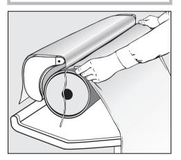
■ Insert the long edge of the new ironing cover into the retaining slot with the side seams inside (upside down). Keep side ties hanging free and smooth out.
