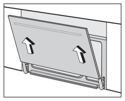
■ While holding the door with both hands, lift the door until the hinges disengage. Remove the door.
