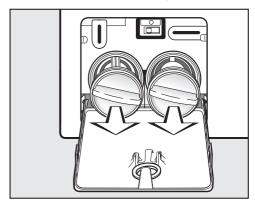
■ Remove the drain filters completely.
