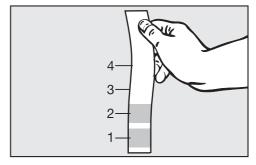
■ Dip the test strip in the water for approx. 1 second. Shake excess water off the test strip.
