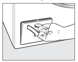
Open the drain pump flap.
