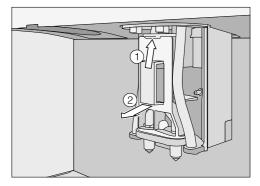
■ Press the catch upwards ①, grasp the dispensing unit by the handle, and pull it forwards and off ②.
