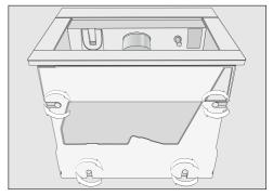
■ Using the large hex key, unscrew all four feet on the underside of the appliance by about 3/4" (2 mm).
