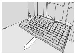
Open the machine front and carefully remove the drip tray from the machine.
