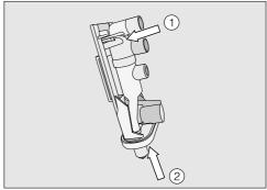
■ Reassemble the dispensing unit in the reverse order. Make sure that upper adapter ① clicks into position. Press the dispenser nozzles ② firmly onto the dispensing unit.
