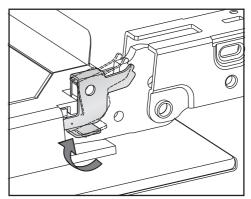
To relock the locking clamps, turn them back up to the horizontal position as far as they will go. The following faults can be corrected without contacting the Miele Service Department.
